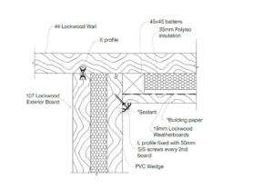
Fix A Corner Profiles by pre-drilling then screwing every second board.
