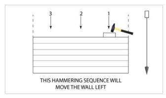
Take your time when there are multiple profiles in a small area, such as stiffener posts between windows, to avoid damaging boards.
