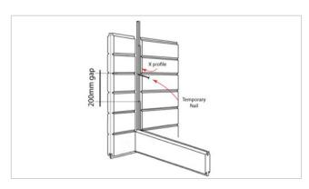
Continually check the walls stay level and plumb as you build and ensure V grooves line up in corners.
