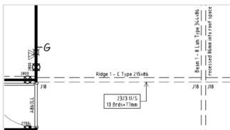
For beams fixed to posts, refer to the Lockwood factory floor plan for the floor to underside of beam measurement. Mark the position of beam on the posts and router out for the beam bracket.
