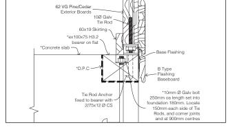
Install DPC in recesses and around the perimeter before installing first boards and full height joinery.
