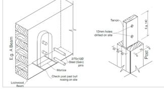
Fit the 'E' beams to interior walls. E beams will all be numbered on the plans. They are supplied approximately 50mm longer than necessary. Trim to correct size before installing.
