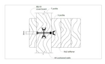
Build up the interior walls locking each into place using a 3-4kg hammer and striker board using an alternating sequence as described on page 15.
