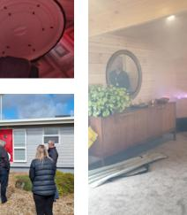
Our designed passive ventilation at the window and door heads are working as intended; faint tendrils of fog could be seen passing through and out under the exterior head flashings.
