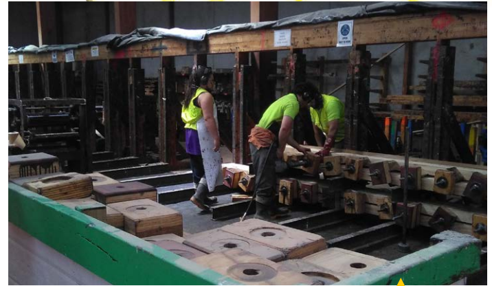
TimberLab staff creating laminated beams ▲
